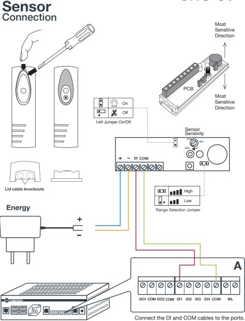
Connect the DI and COM cables to the ports. You can connect the end of the DI Cable to any of the Digital Inputs.
