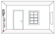
To be able to operate the sensor efficiently, the height of the installation site should be 2.20m - 2.70m.
