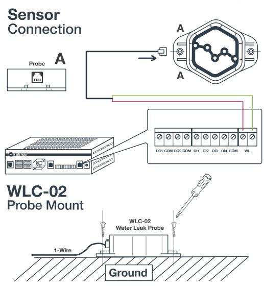
It is important to install the water leak sensor probe where water leakage may occur. For example: In data centers, server rooms can be installed on the floor below. The place to be installed must be free from dust.
